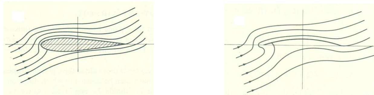
Figure 3: An object with an aerofoil shaped cross-section; left : symmetric aerofoil with flow at an angle of attack; right : circular arc aerofoil of zero thickness.
