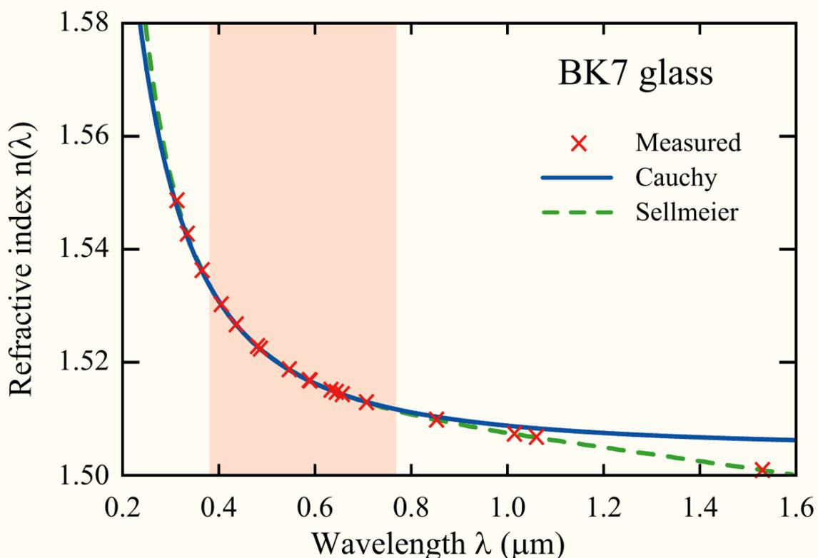
Refractive index vs. wavelength for BK7 glass. Red crosses show measured values. Over the visible region (red shading), Cauchy's equation (blue line) agrees well with the measured refractive indices and the Sellmeier plot (green dashed line). It deviates in the ultraviolet and infrared regions.
