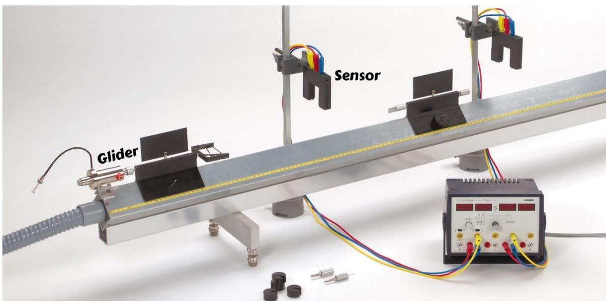
Learn how to use the sensor-timer to measure the velocity of the glider going through the sensor. There are two sensors and four displays on the timer. Two of the displays measure the time of the first pass and the second pass of an object through the first sensor.
