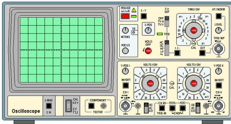
In the dual beam CRO two electron beams are obtained in the CRT. The beams produce two spots of light on the CRT screen and facilitate simultaneous observation of two signal waveforms.
