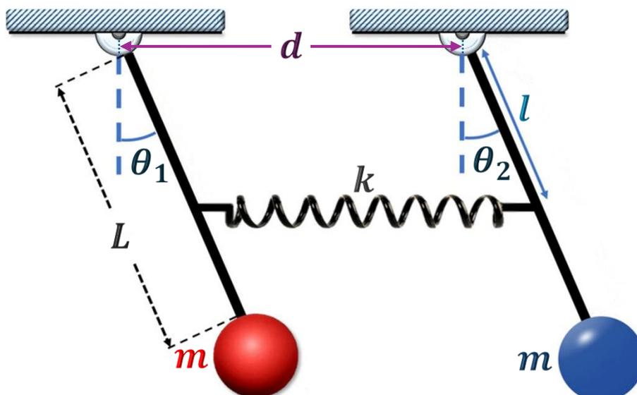
**Fig. 1** – Schematic of coupled pendula with coupling spring attached at the end.
