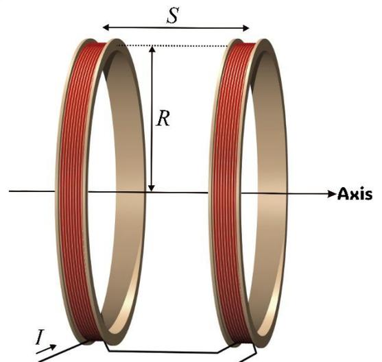
Because of these properties, the axial magnetic field is fairly constant over a certain region in the middle of the pair of coils. This arrangement is very popular in producing uniform axial fields in regions easily accessible to experimental situations needing such uniformity.
